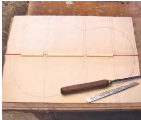
STEP 22. The cross-banding to strengthen the join in the back
